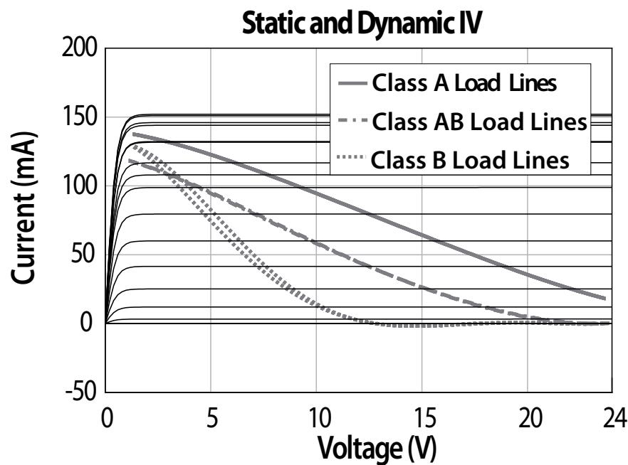
Figure 5.21: Variation of the dynamic load lines at the fundamental frequency for the active devices of a CRLH-TL-based distributed amplifier working under different modes of operation (A, AB and B).
