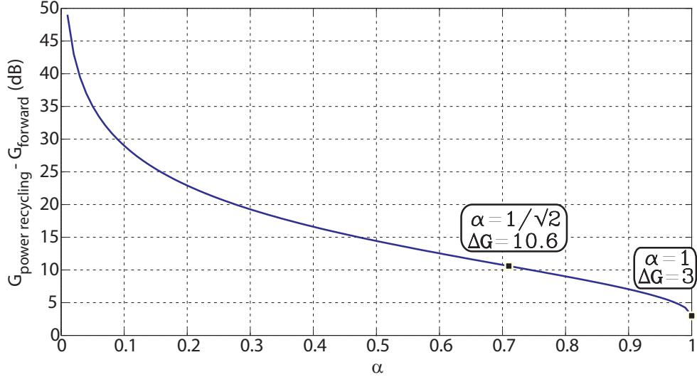
Figure 3.2: Gain increase of the power recycling distributed amplifier in respect to the forward gain of the single-fed configuration as a function of the degree of coupling of the input directional coupler ( $A$ ) for a single frequency (optimum phase conditions for the maximization of the gain)
