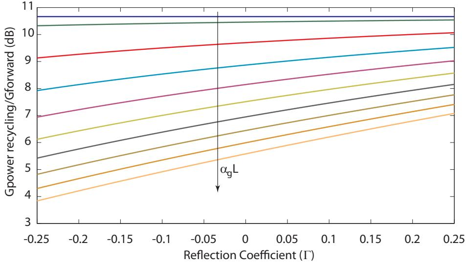
Figure 3.5: Power recycling distributed amplifier gain enhancement versus the forward gain of a generic distributed amplifier (3dB directional coupler-based implementation) as a function of  $\Gamma$  and  $\alpha_{g\_line}L$  ( $\theta_{g\_line} + \theta_{aux1} + \theta_{aux2} = \frac{3\pi}{2}$ ,  $\alpha_{g\_line}L = [0, 0.01, 0.05, 0.1, 0.15, \dots, 0.4]$ )
