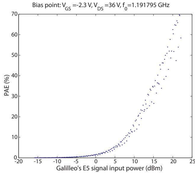
Figure C.11: Measured PAE under Galileo's E5 modulated signal. Class AB biasing point.
