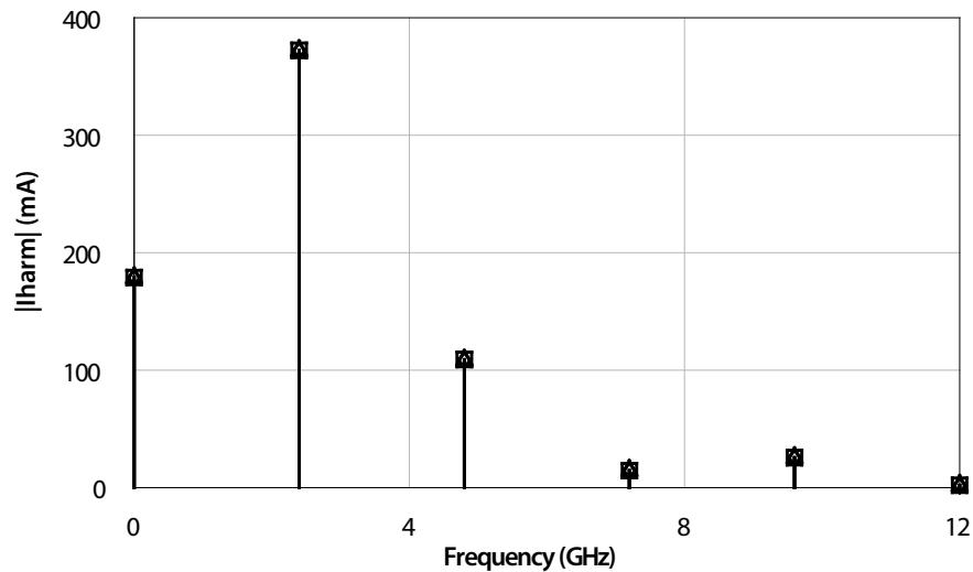
Figure 5.26: Harmonic components for the current for a 3-stage Class AB distributed power amplifier with output power combination ( $P_{in} = 18dBm$ )
