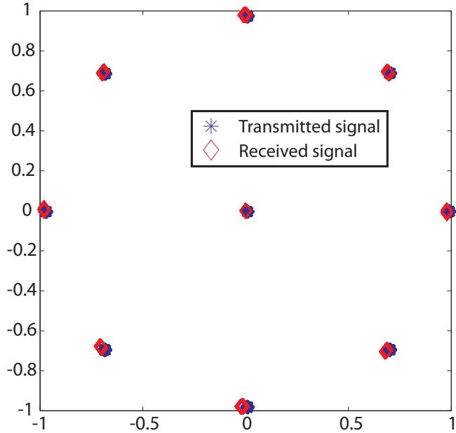
Figure C.7: Normalized Galileo's E5 signal constellation ( $P_{in}=4$  dBm).
