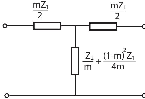
Figure 2.17:  $m$ -derived section with T-topology
