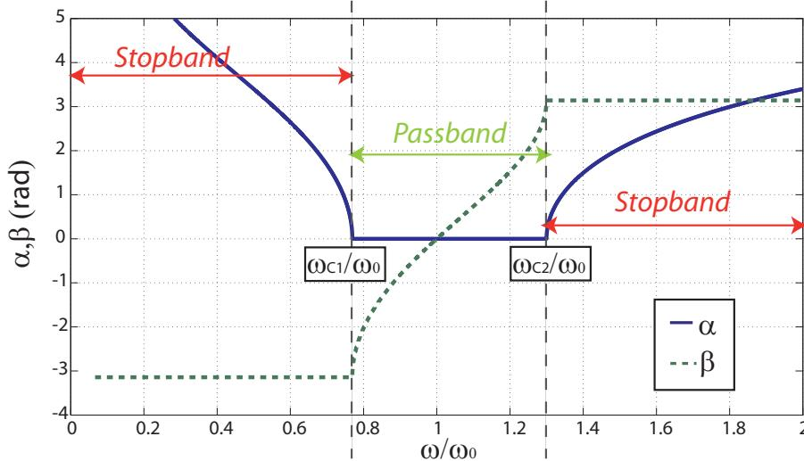
Figure A.6: Propagation constant of a CRLH-TL unit cell
