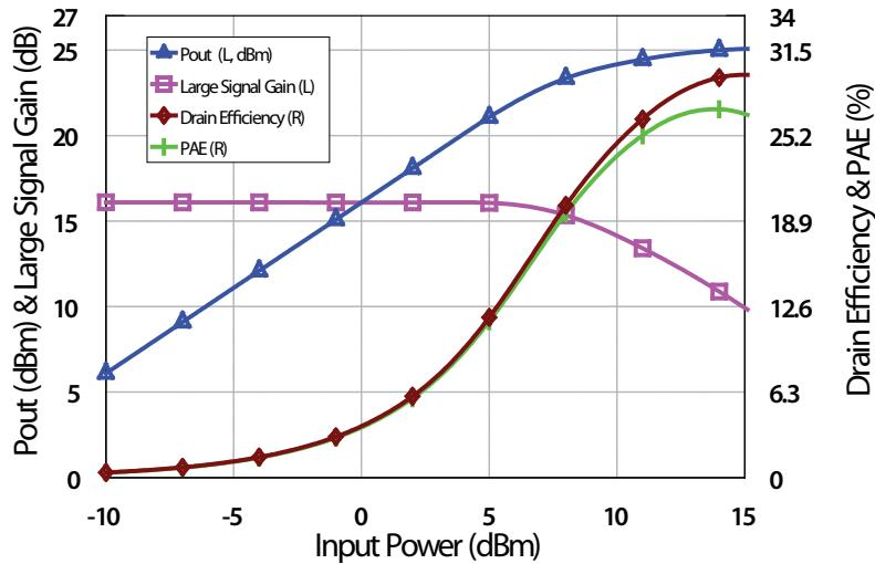
Figure 4.18: Simulated output power (blue), large signal gain (purple), drain efficiency (brown) and PAE (green)  $f_0$ .
