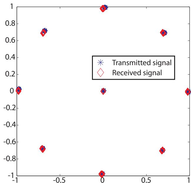
Figure C.12: Normalized Galileo's E5 signal constellation (Pin=24 dBm, Class AB biasing point).
