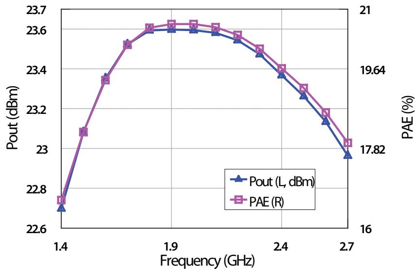
Figure 4.19: Simulated output power (blue), PAE (purple) versus frequency @ CP-1dB=8.5 dBm.
