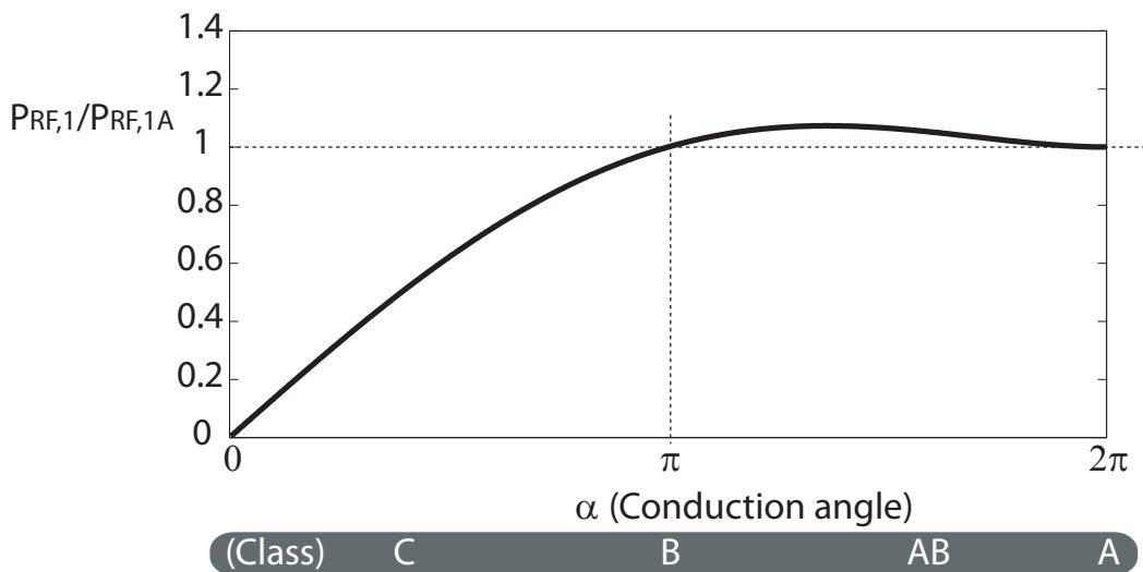
Figure 5.5: Output RF power at the fundamental frequency,  $P_{RF,1}$ , normalized to the corresponding Class A output RF power, as a function of the conduction angle,  $\alpha$ .
