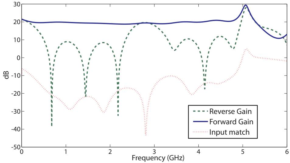
Figure 3.7: Simulated small signal gain (forward and reverse) and input matching for a 4-stage distributed amplifier ( $V_{DS} = 3V, I_{DS} = 20mA$ )
