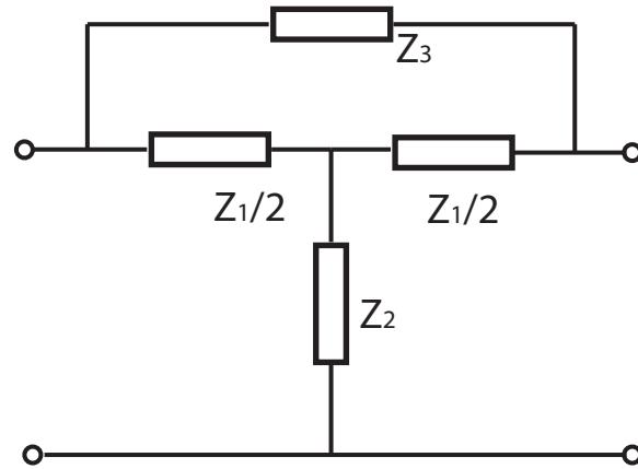
Figure 2.18: Bridged-T section
