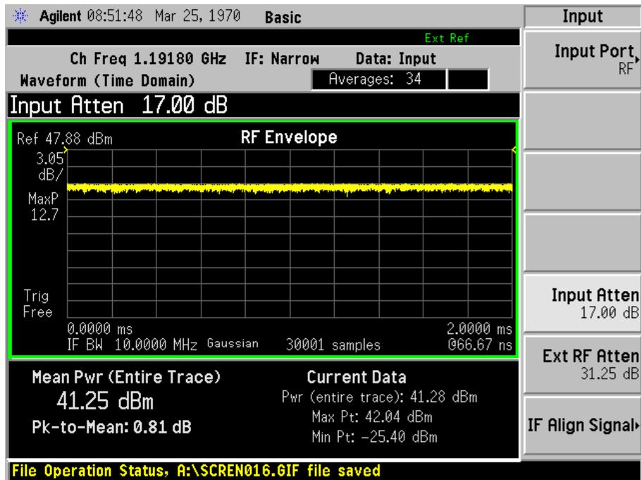
Figure C.9: Amplified E5 signal's envelope (Pin=24 dBm).
