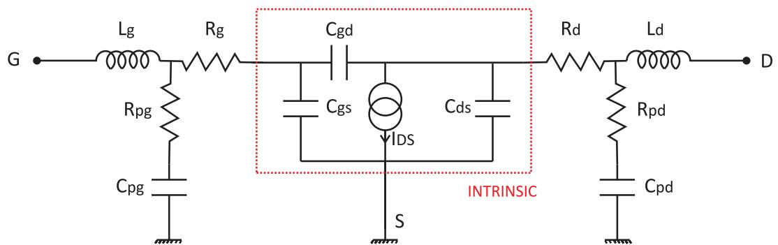
Figure 2.16: Small-signal equivalent circuit for a GaN active device
