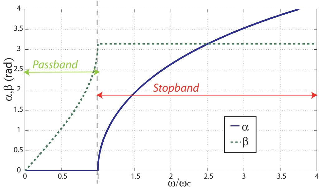
Figure A.2: Propagation constant of a conventional RH-TL unit cell
