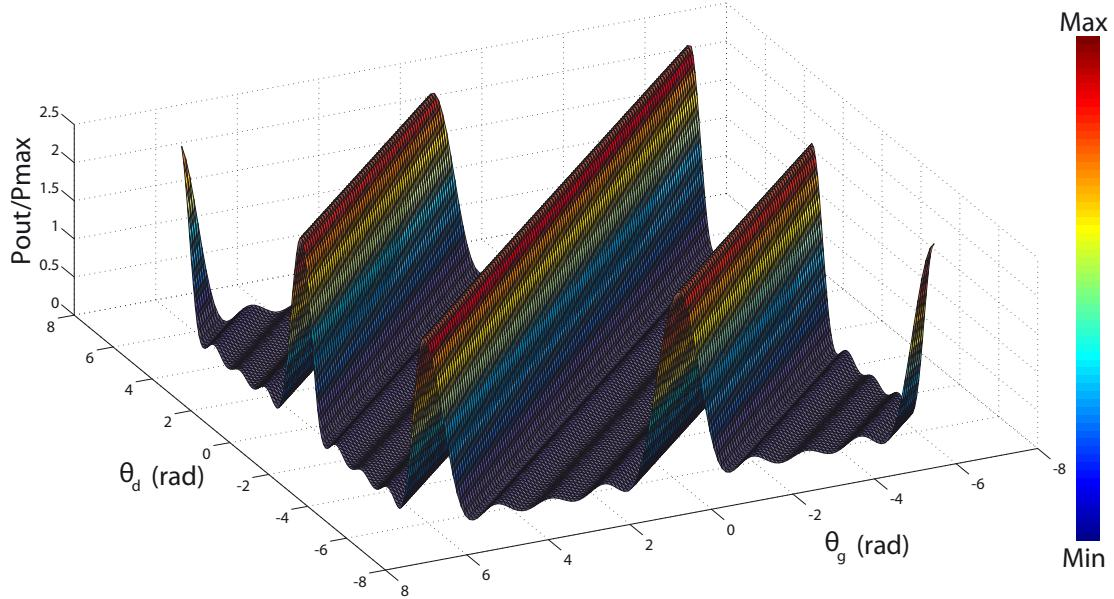
Figure 2.11: Output power at the reverse port for a 5-stage single-fed distributed amplifier as a function of gate and drain phase shifts (red areas represent maximum power values)
