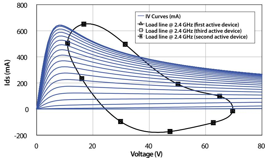
Figure 5.24: IV Curves and Dynamic load lines for a 3-stage Class AB distributed power amplifier with output power combination ( $V_{GS} = [-3 : 0.2 : 2]V$ ,  $P_{in} = 18dBm$ )
