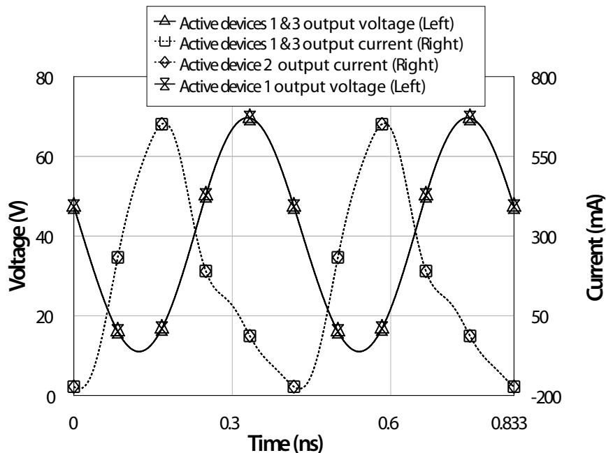
Figure 5.25: Output current and voltage waveforms for 3 active devices of a Class AB distributed power amplifier with output power combination @  $f_0$  ( $P_{in} = 18dBm$ )
