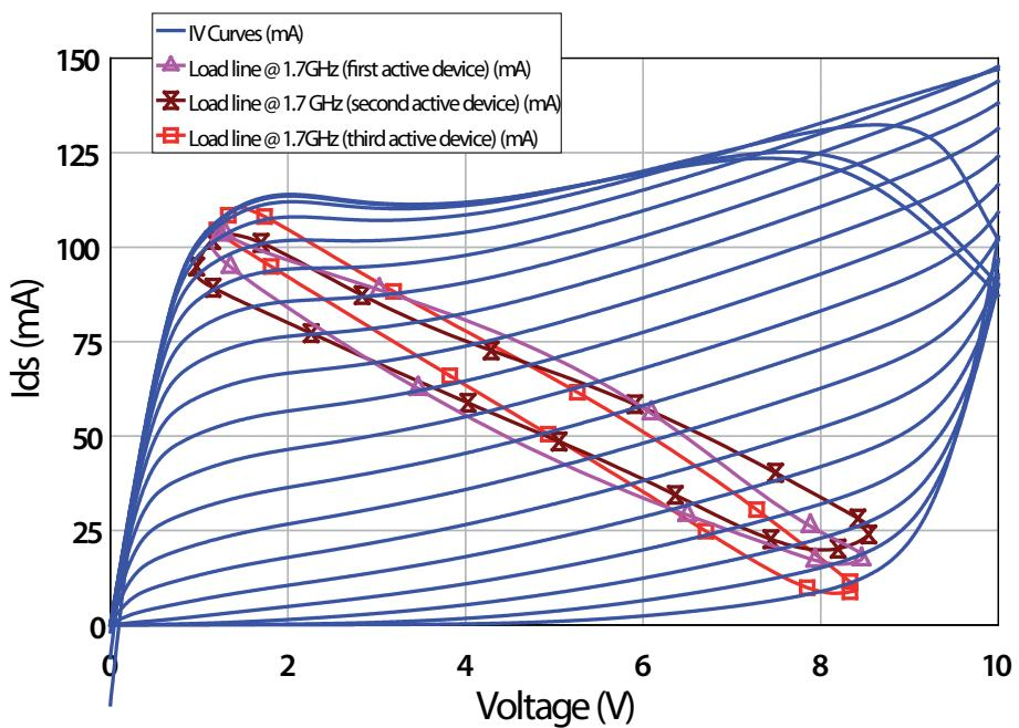
Figure 4.20: Load lines for the three active devices @ 1.7 GHz for the CP-1dB.
