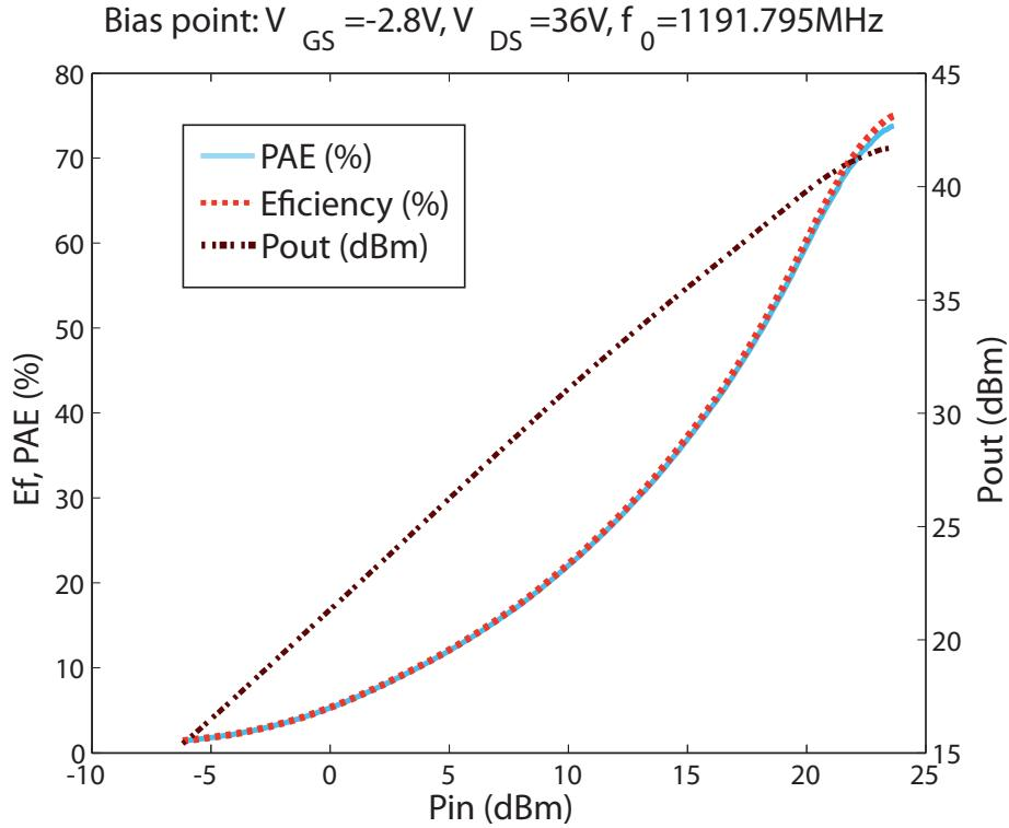
Figure C.3: Measured output power, efficiency and PAE.
