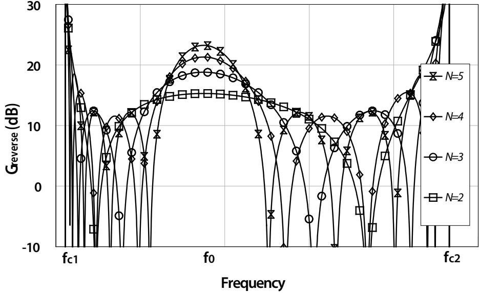
Figure 2.4: Reverse gain of a CRLH-TL-based distributed amplifier for a different number of amplifier stages
