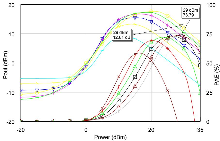
Figure C.17: Simulated gain and PAE versus input power for different  $V_{DS}$  values at the fundamental frequency of 3.5 GHz
