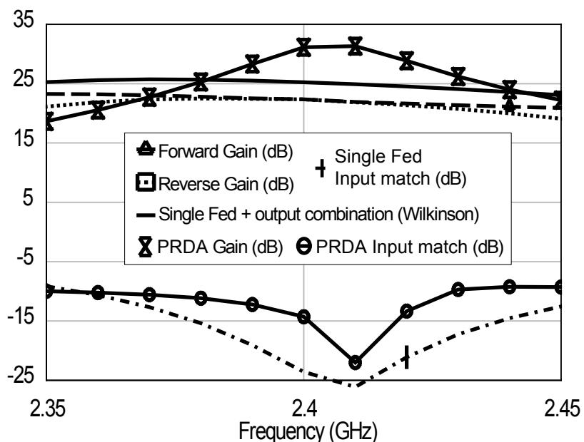
Figure 5.29: Simulated small-signal S-parameters of a 3-stage CRLH-TL-based power recycling distributed power amplifier working under Class AB
