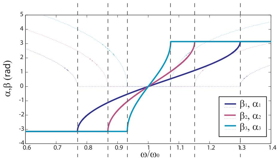
Figure A.10: Propagation constants ( $\beta$ : full line,  $\alpha$ : dotted line) for a balanced CRLH-TL unit cell with three different slopes
