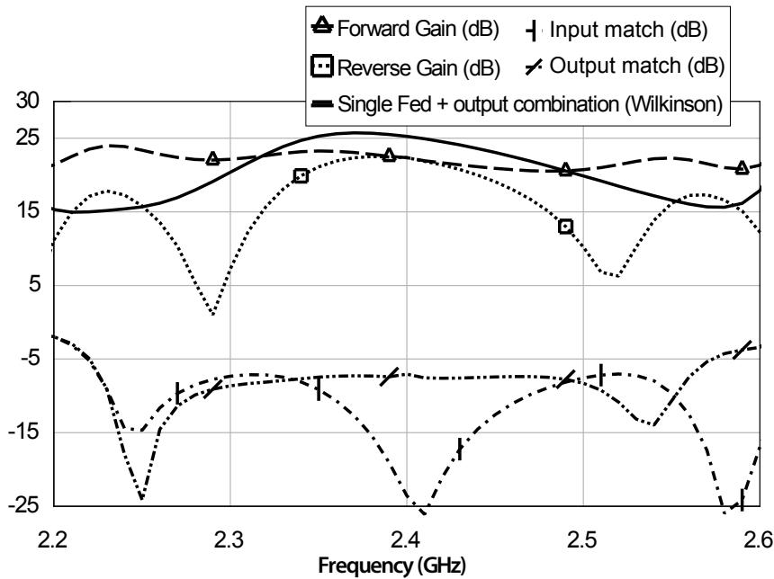
Figure 5.23: Simulated S-parameters of a 3-stage CRLH-TL-based distributed power amplifier working under Class AB
