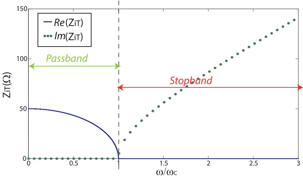
Figure A.4: Image impedance of a conventional RH-TL unit cell with  $T$ -topology
