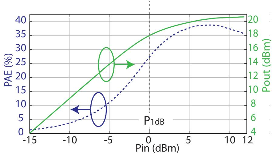
Figure 4.11: Measured power added efficiency (dashed line) and output power (solid line) for the 3-stage CRLH-TL-based power recycling distributed amplifier ( $I_{DS} = 30mA$ ;  $V_{DS} = 3V$ ) @  $f_0 = 1.07GHz$
