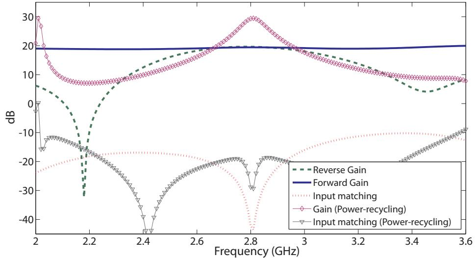
Figure 3.9: Simulated small signal gain (forward and reverse) and input matching for a 4-stage distributed amplifier in single-fed and power recycling (3dB 180° hybrid-based) configuration ( $V_{DS} = 3V, I_{DS} = 20mA$ )
