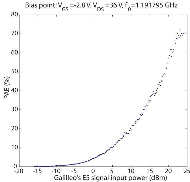
Figure C.6: Measured PAE under the Galileo's E5 modulated signal.
