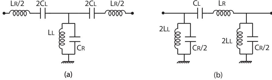
Figure A.5: CRLH unit cell with (a)  $T$ - and (b)  $\pi$ -topology
