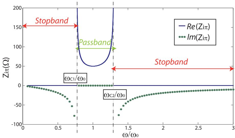
Figure A.7: Image impedance of a CRLH-TL unit cell with  $\pi$ -topology
