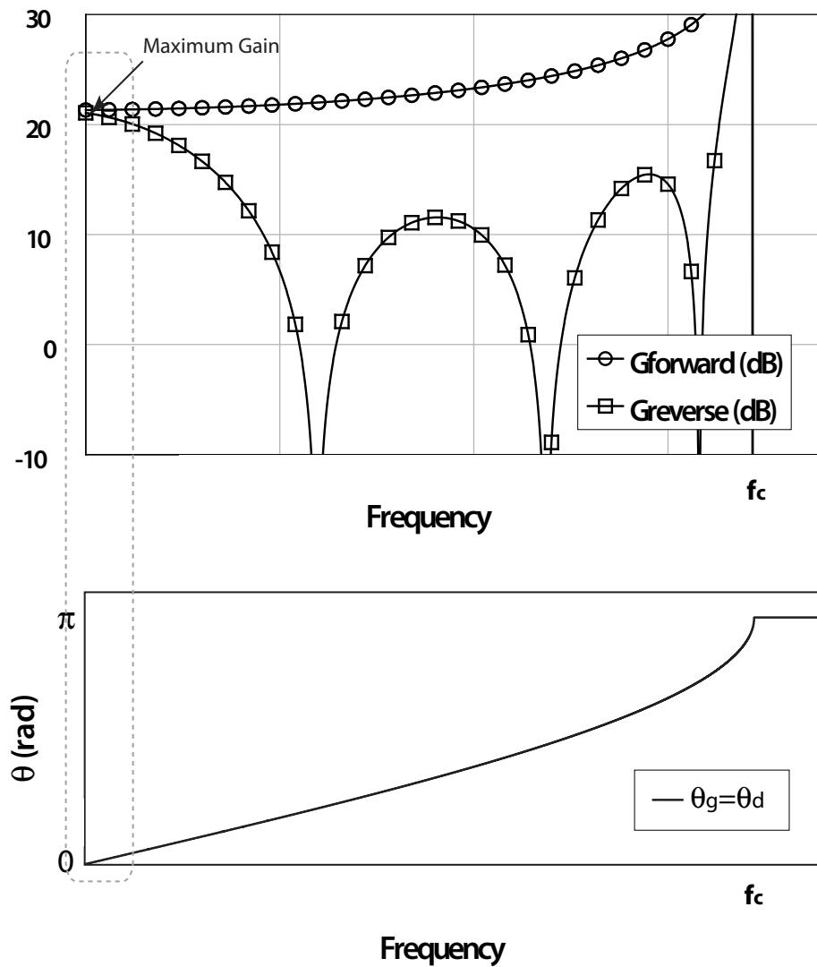
Figure 2.5: Forward and reverse gain of a 4-stage RH-TL-based distributed amplifier with identical gate and drain phase constants
