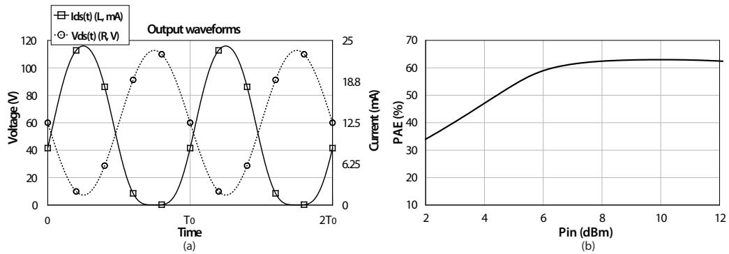
Figure 5.19: Theoretical output waveforms (a) and power added efficiency (b) for a Class AB distributed power amplifier @  $f_0$  ( $I_{DS} = 41.5\text{mA}$ ,  $V_{DS} = 12.5\text{V}$ ).
