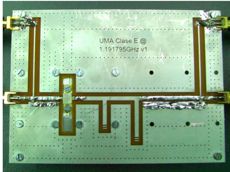
Figure C.1: Class E GaN HEMT amplifier prototype
