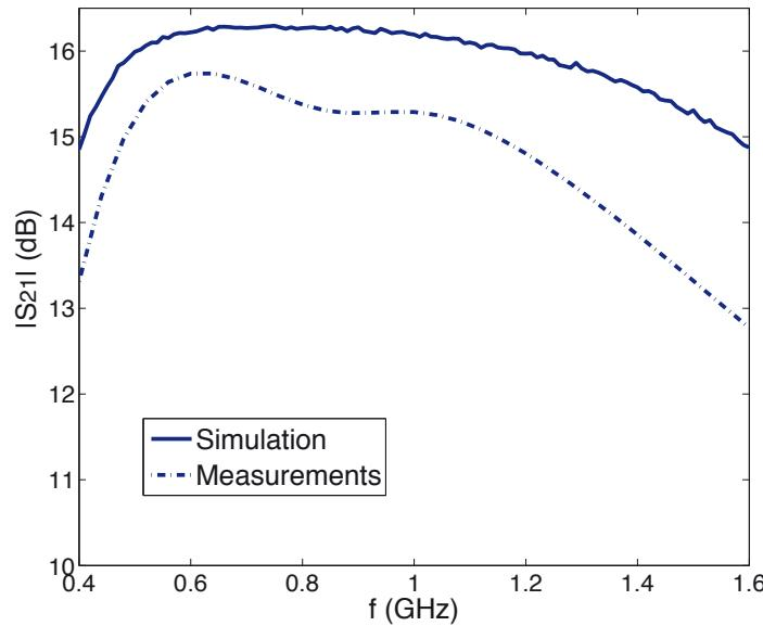
Figure 4.1: Small Signal Gain for a 3-stage CRLH-TL-based dual-fed distributed amplifier ( $V_{GS} = -0.3V, V_{DS} = 3V$ )
