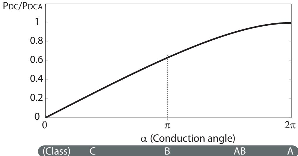
Figure 5.4: DC power,  $P_{DC}$ , normalized to the corresponding Class A DC power consumption, as a function of the conduction angle,  $\alpha$ .
