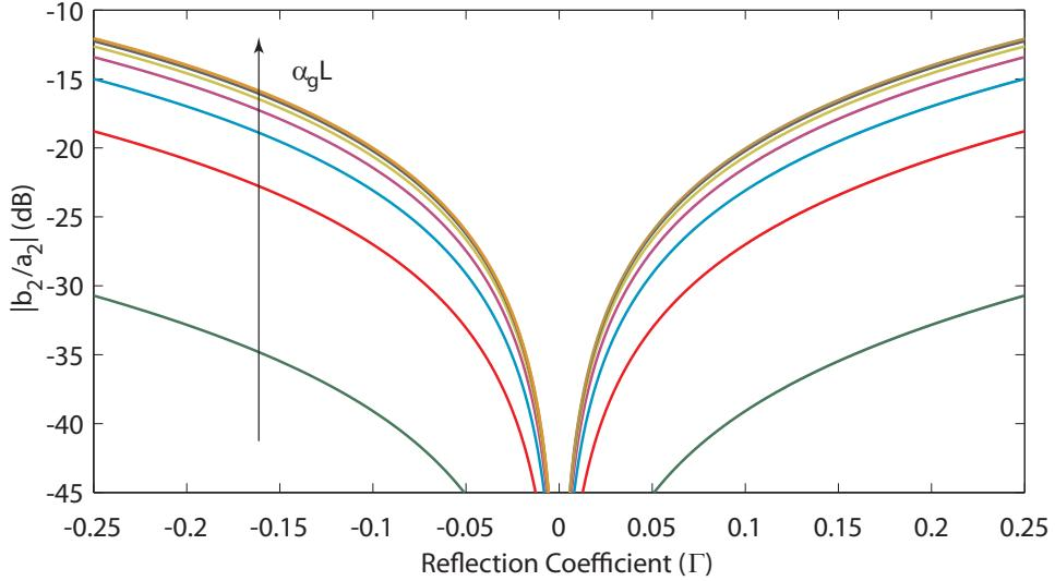
Figure 3.4: Input matching simulation for the power recycling distributed amplifier (3dB directional coupler-based implementation) as a function of  $\Gamma$  and  $\alpha_{g.line}L$  ( $\theta_{g.line} + \theta_{aux1} + \theta_{aux2} = \frac{3\pi}{2}$ ,  $\alpha_{g.line}L = [0.01, 0.05, 0.1, 0.15, \dots, 0.4]$ )
