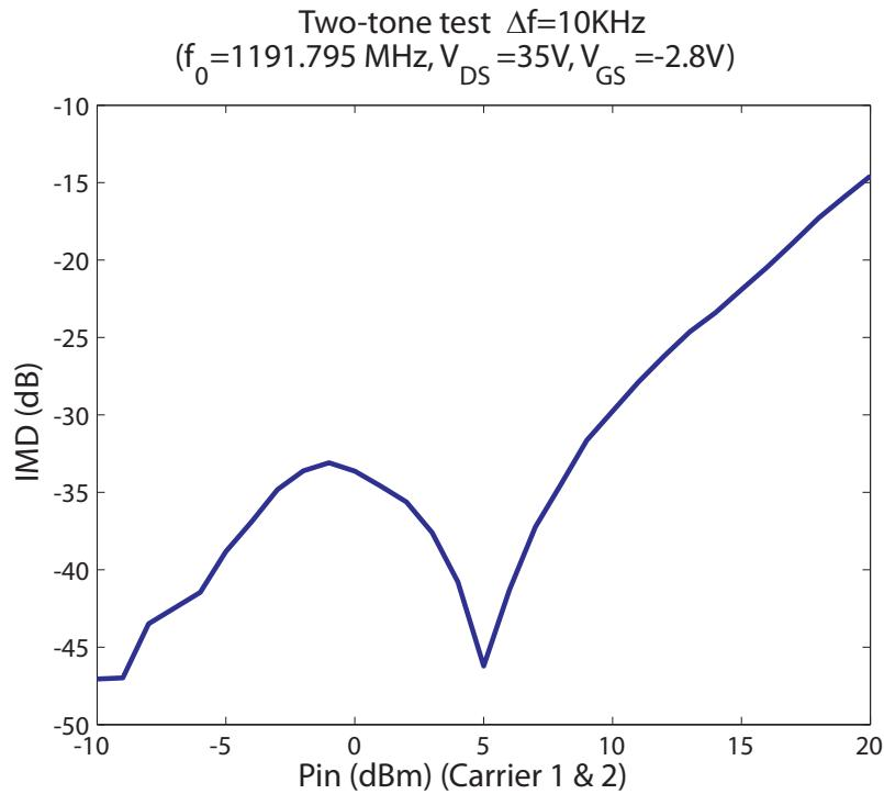
Figure C.4: Measured intermodulation distortion.
