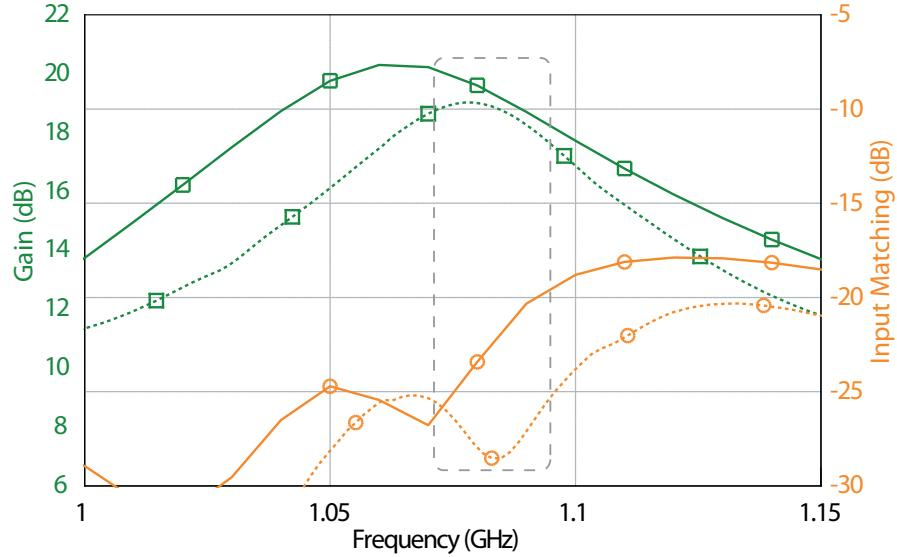
Figure 4.9: Simulated (solid line) and measured (dashed line) small signal gain and input matching for a 3-stage power recycling CRLH TL-based distributed amplifier ( $I_{DS} = 30mA$ ;  $V_{DS} = 3V$ )
