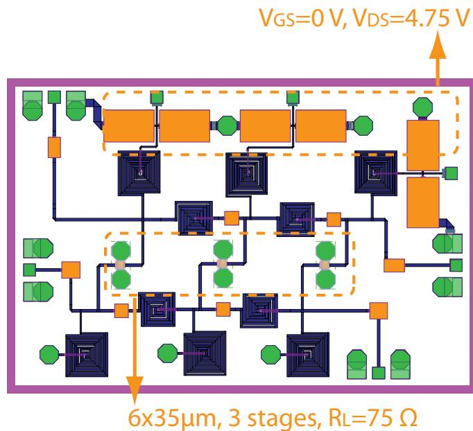
Figure 4.16: Distributed amplifier's layout (access ports highlighted).
