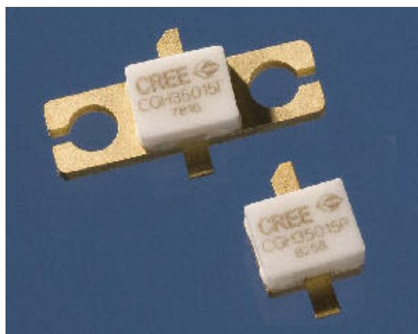
Figure C.13: CGH35015 GaN transistor
