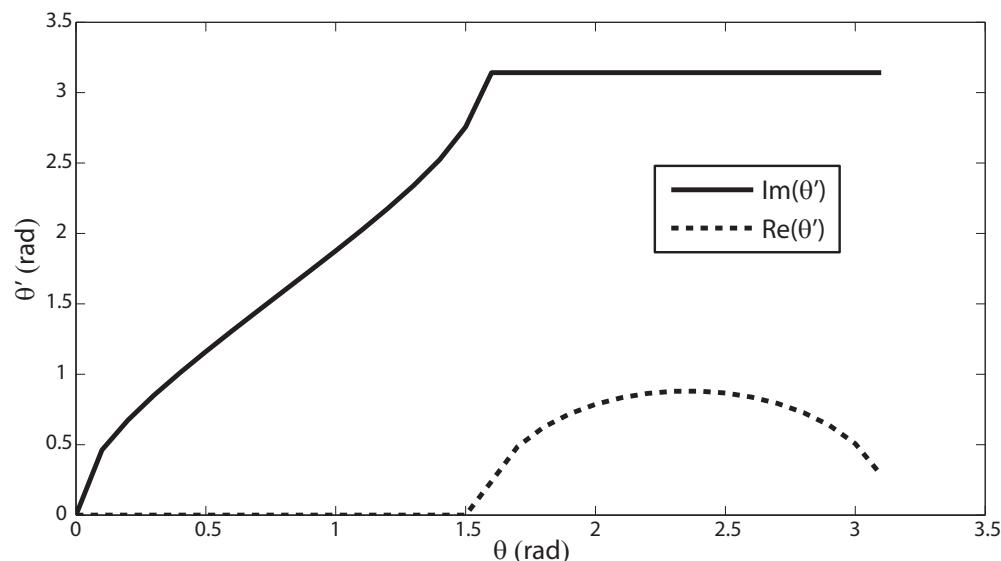
Figure A.13: Dispersion diagram for a lossless transmission line periodically loaded with a capacitance ( $\bar{y} = j$ , imaginary part in full line and real part in dashed line).
