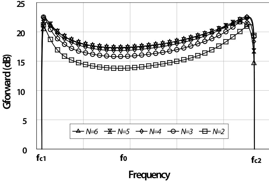
Figure 2.14: Effect of losses ( $\alpha = 1.5\text{dB}$  per stage) on the forward gain of a CRLH-TL-based distributed amplifier as a number of amplifier stages
