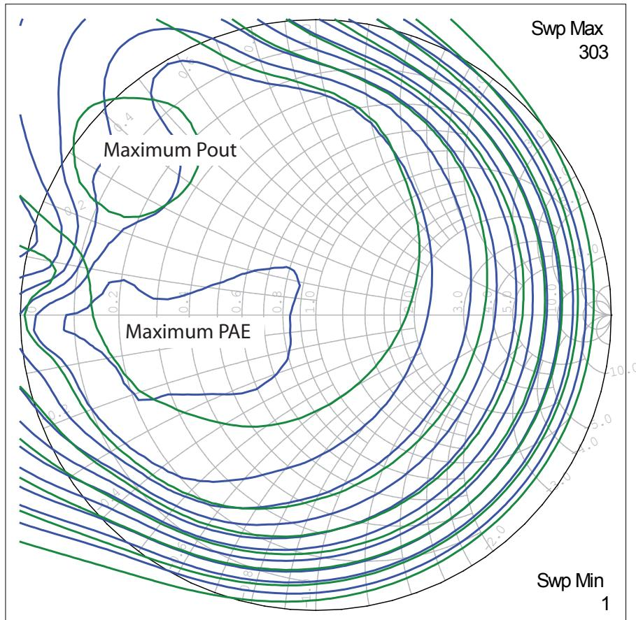
Figure 5.7: Simulated load pull output power and efficiency contours for a GaN HEMT (Cree, CGH35015F) at the fundamental load of 900MHz.
