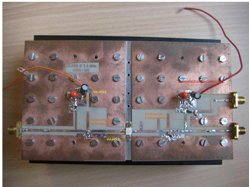
Figure C.19: Class E power amplifier for 3.5 GHz
