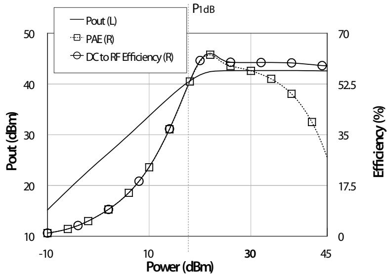
Figure 5.28: Output power and Power added efficiency of a 3-stage Class AB distributed power amplifier with output power combination
