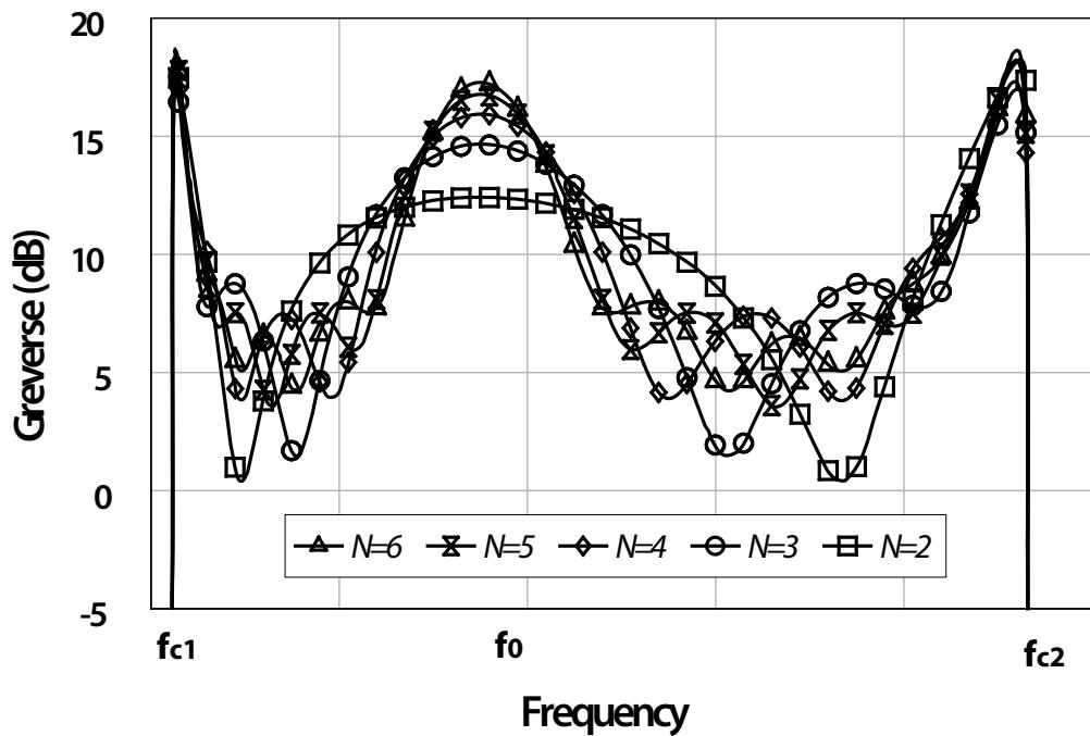
Figure 2.15: Effect of losses ( $\alpha = 1.5\text{dB}$  per stage) on the reverse gain of a CRLH-TL-based distributed amplifier as a number of amplifier stages
