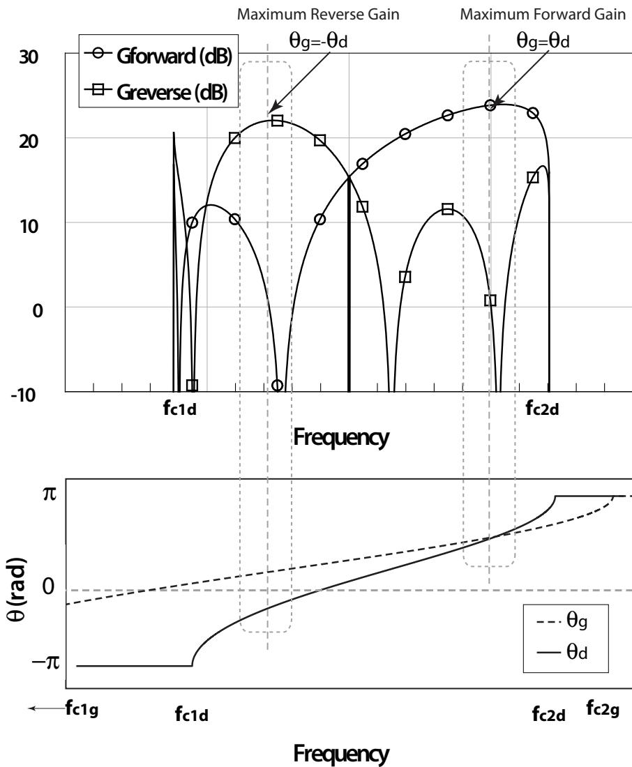
Figure 2.7: Forward and reverse gain of a 4-stage CRLH-TL-based distributed amplifier with different gate and drain phase constants
