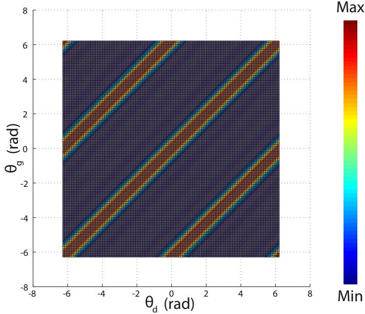
Figure 2.10: Output power at the forward port for a 5-stage single-fed distributed amplifier as a function of gate and drain phase shifts (red areas represent maximum power values)
