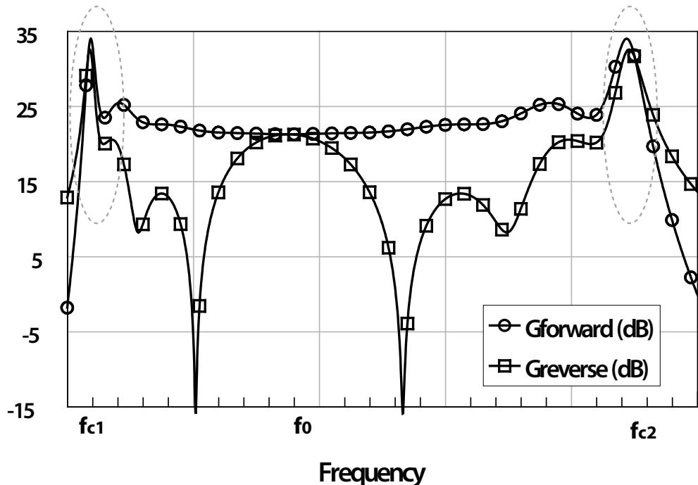
Figure 2.19: Forward and reverse gain of a 4-stage CRLH-TL-based distributed amplifier with identical phase constants terminated with an  $50\Omega$  load impedance
