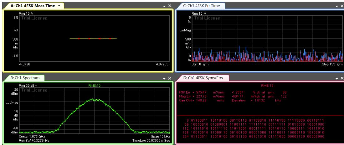
Figure 4.13: Amplified 4FSK signal @ P1dB
