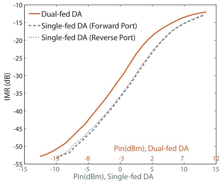
Figure 4.5: Measured Intermodulation Distortion Ratio @ 1 GHz ( $V_{GS} = -0.3V$ ,  $V_{DS} = 3V$ , two-tone test  $\Delta f = 1MHz$ )
