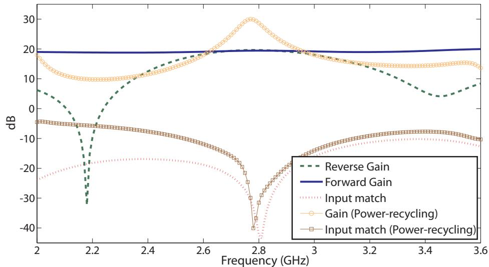
Figure 3.10: Simulated small signal gain (forward and reverse) and input matching for a 4-stage distributed amplifier in single-fed and power recycling (3dB 90° hybrid-based) configuration ( $V_{DS} = 3V, I_{DS} = 20mA$ )
