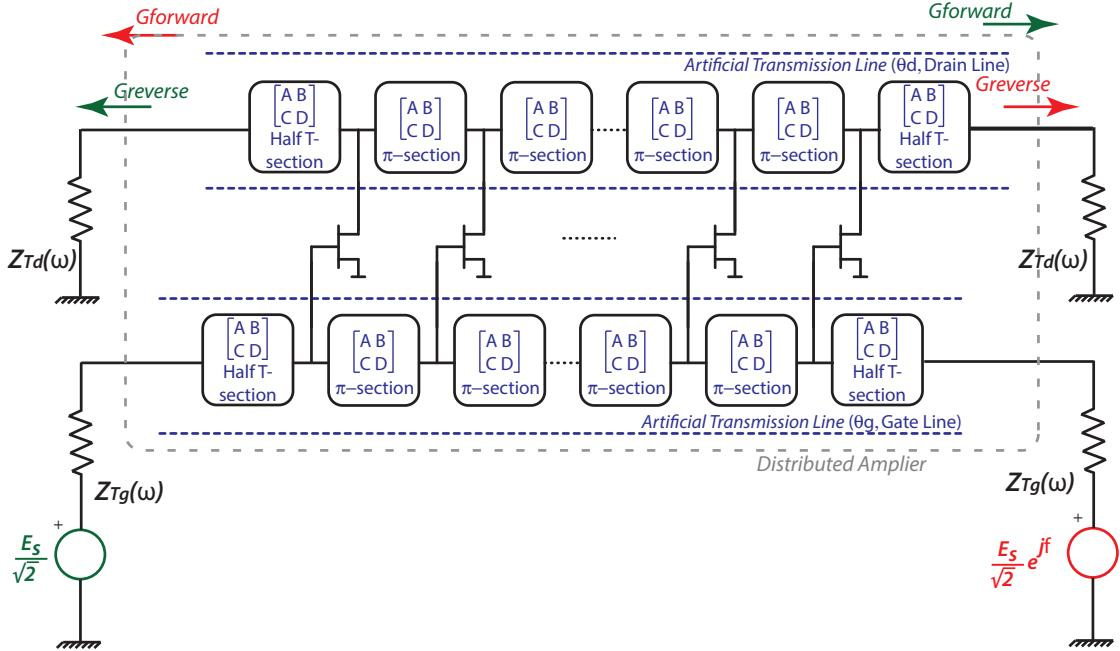
Figure 2.13: Generic dual-fed distributed amplifier equivalent circuit
