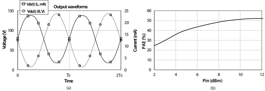
Figure 5.18: Theoretical output waveforms (a) and power added efficiency (b) for a Class A distributed power amplifier @  $f_0$  ( $I_{DS} = 79.5\text{mA}$ ,  $V_{DS} = 12.5\text{V}$ ).
