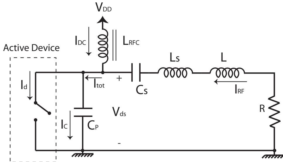
Figure 5.10: Circuit topology for a Class E power amplifier
