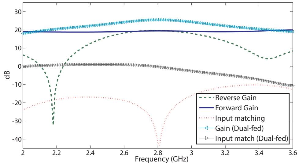
Figure 3.8: Simulated small signal gain (forward and reverse) and input matching for a 4-stage distributed amplifier in single- and dual-fed configuration ( $V_{DS} = 3V, I_{DS} = 20mA$ )
