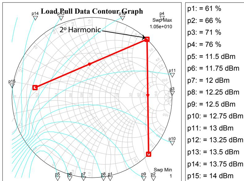
Figure C.15: Simulated load pull output power (blue) and efficiency (gray) contours for a GaN HEMT (Cree, CGH35015F) at the second harmonic.
