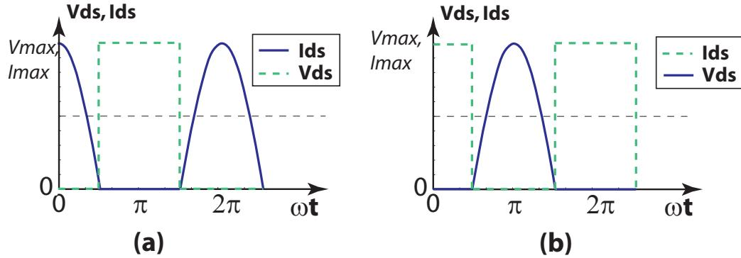
Figure 5.8: Drain voltage and drain current waveforms for a infinite order Class F (a) and a Class  $F^{-1}$  (b) power amplifier
