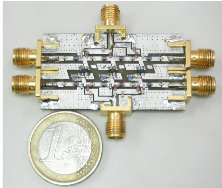
Figure 4.7: CRLH TL-based distributed amplifier prototype (hybrid technology)
