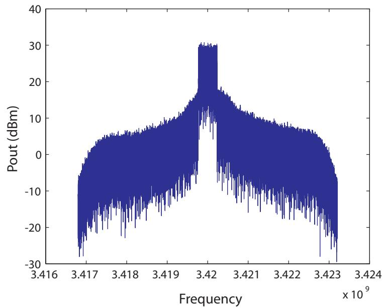
Figure C.21: Output power spectrum for a WiMAX signal (500kHz bandwidth) versus frequency for a 29.69 dBm input power
