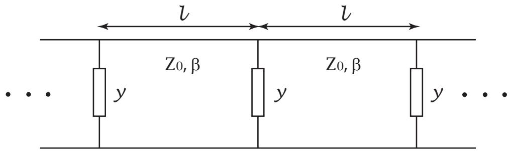
Figure A.11: Periodically loaded transmission line
