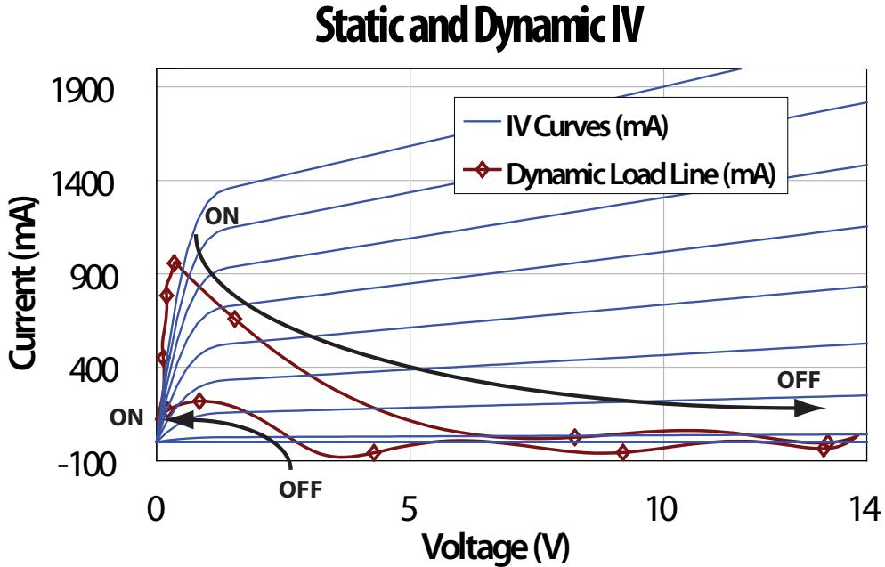
Figure 5.12: Class E amplifier load curve
