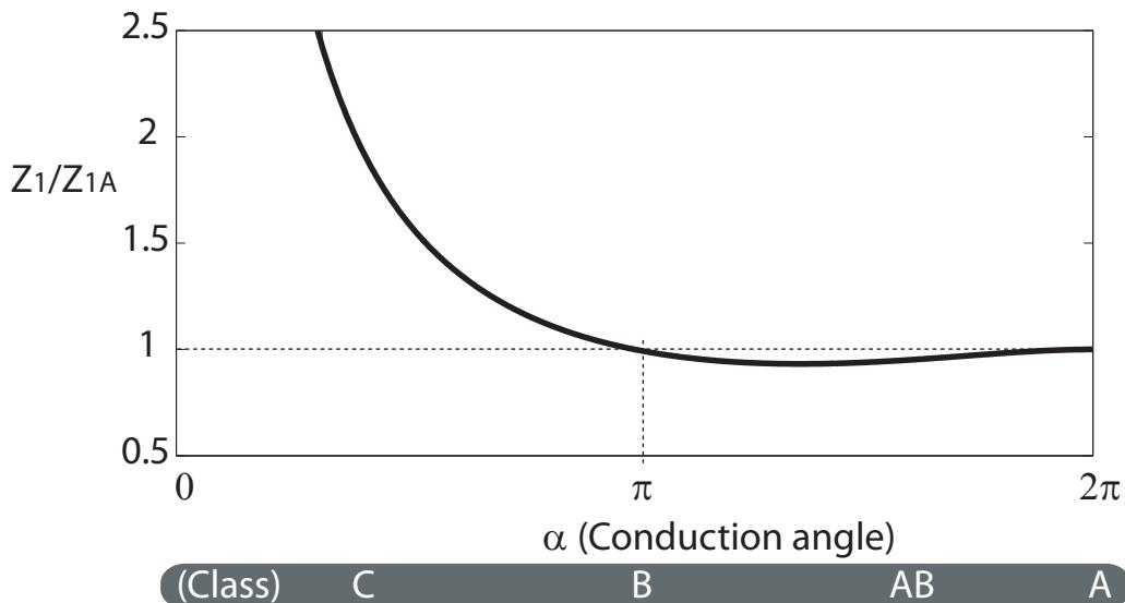
Figure 5.3: Optimum load for the fundamental frequency,  $Z_1$ , normalized to the corresponding Class A optimum load, as a function of the conduction angle,  $\alpha$ .
