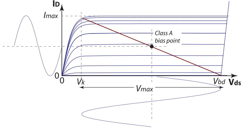
Figure 2.8: Optimum Class A load line for maximum voltage and current excursion
