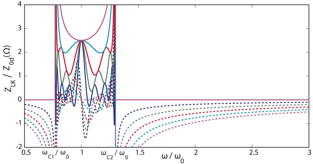
Figure 5.13: Load impedances for a 5-stage CRLH-TL-based single-fed distributed amplifier as function of the normalized frequency (real part in full line and imaginary part in dashed line)
