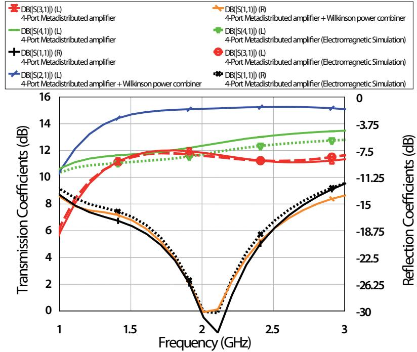
Figure 4.17: Circuitual (solid line) and electromagnetic (dashed line) S-parameters simulation.
