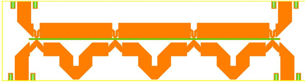
Figure 3.6: Layout for the designed distributed amplifier
