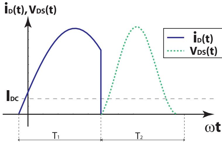
Figure 5.11: Ideal normalized Class E output current and voltage waveforms
