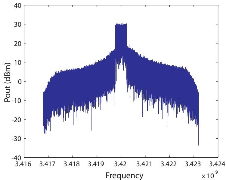
Figure C.22: Output power spectrum for a WiMAX signal (500kHz bandwidth) versus frequency for a 31.47 dBm input power
