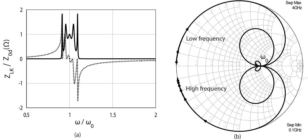
Figure 5.17: (a) Load impedance CRLH-TL-based single-fed distributed amplifier as function of the normalized frequency (real part in full line and imaginary part in dashed line). (b) Load impedance representation in the Smith Chart.
