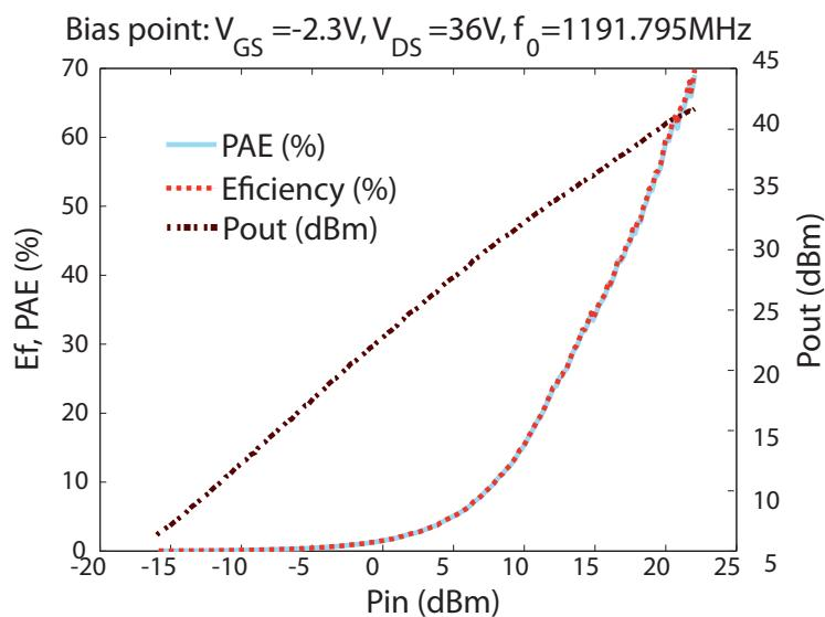
Figure C.10: Measured output power, efficiency and PAE. Class AB biasing point.
