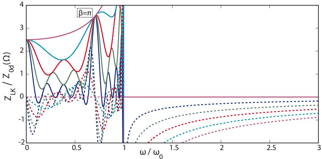
Figure 5.14: Load impedances for a 5-stage RH-TL-based single-fed distributed amplifier as function of the normalized frequency (real part in full line and imaginary part in dashed line)
