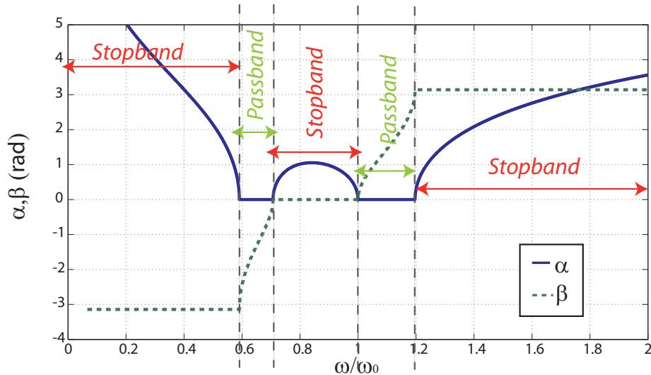
Figure A.9: Propagation constant of an unbalanced CRLH-TL unit cell
