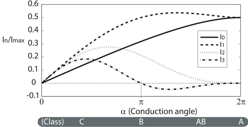
Figure 5.2: Fourier coefficients normalized to the device maximum current,  $I_{max}$ , as a function of the conduction angle,  $\alpha$ .
