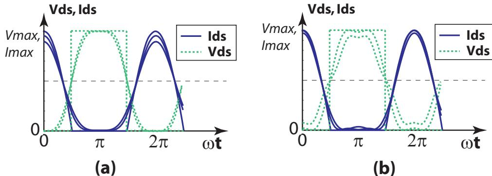
Figure 5.9: Drain voltage and drain current waveforms for a finite order Class F power amplifier with maximally flat drain-to-source voltage and a finite order Class F power amplifier with maximum drain efficiency compared to an infinite order Class F
