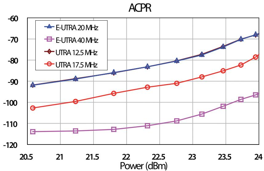
Figure 4.22: Simulated ACPR for different interfering channels for an LTE FDD signal @ 1.9 GHz.
