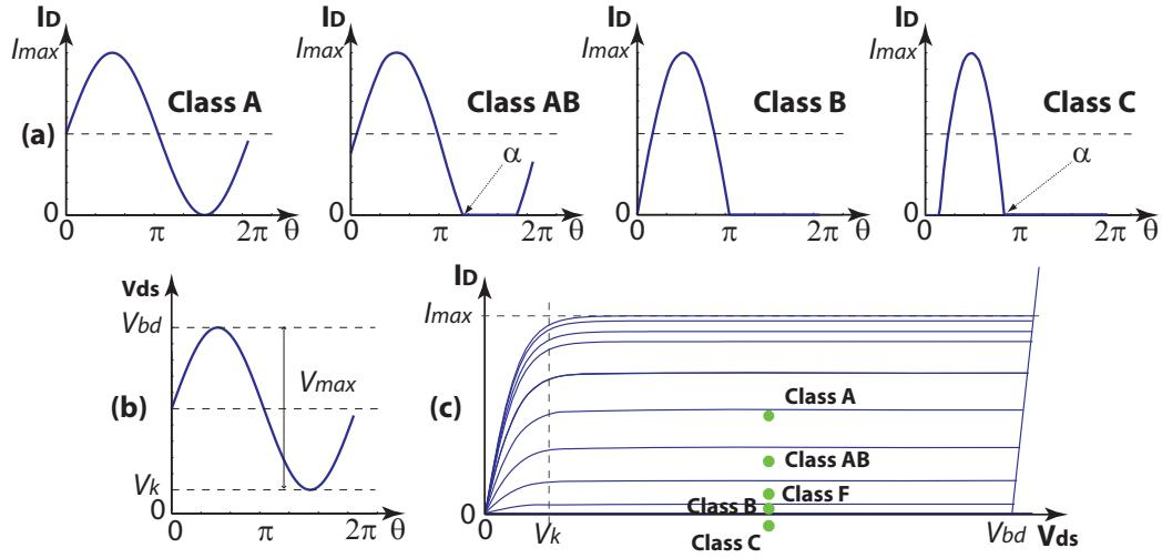
Figure 5.1: Current (a) and voltage (b) waveforms, and bias points (c) for the conventional high efficiency amplifier modes.
