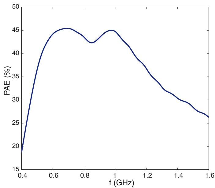
Figure 4.4: Measured Power Added Efficiency versus frequency for a 3-stage CRLH-TL-based dual-fed distributed amplifier ( $V_{GS} = -0.3V, V_{DS} = 3V, Pin = 11.5dBm$ )
