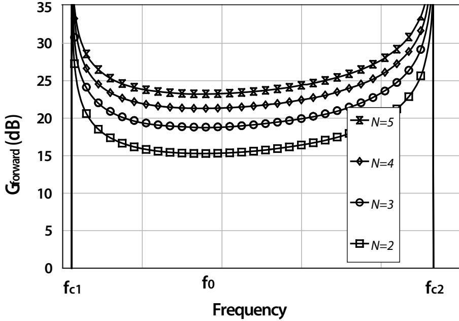
Figure 2.3: Forward gain of a CRLH-TL-based distributed amplifier for a different number of amplifier stages ( $f_{c1}$ ,  $f_{c2}$  cutoff frequencies)
