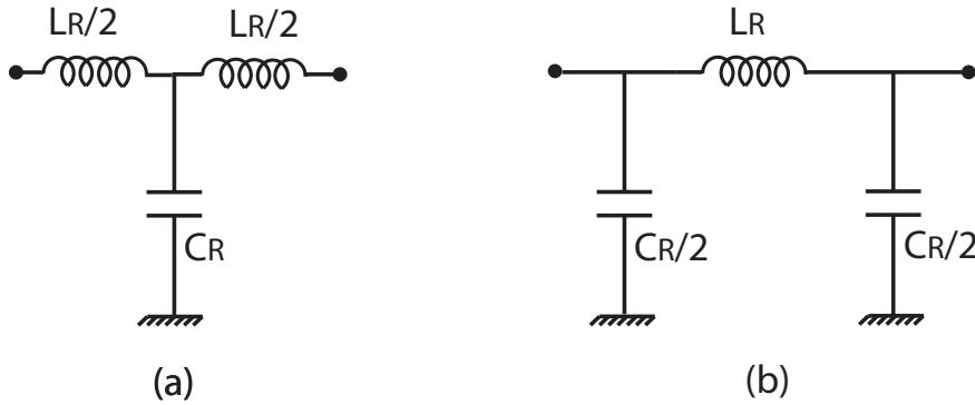
Figure A.1: Conventional RH unit cell with (a)  $T$ - and (b)  $\pi$ -topology
