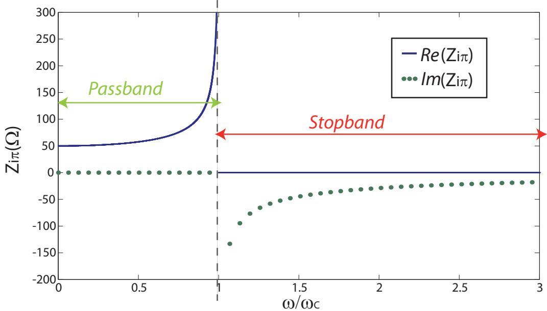
Figure A.3: Image impedance of a conventional RH-TL unit cell with  $\pi$ -topology
