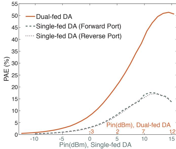
Figure 4.3: Measured Power Added Efficiency @ 1 GHz ( $V_{GS} = -0.3V, V_{DS} = 3V$ )
