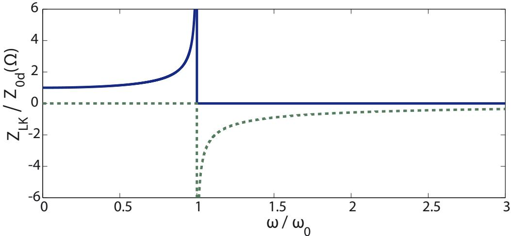
Figure 5.16: Image impedance of the drain unit cell (RH-TLs) with  $\pi$ -topology
