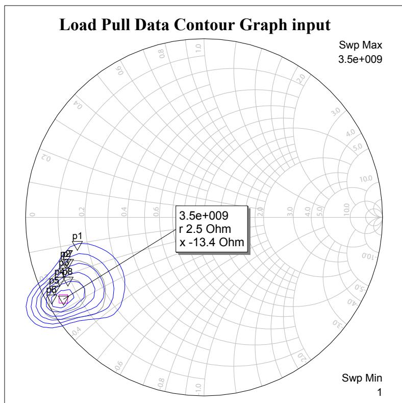
Figure C.16: Simulated load pull gain (gray) and efficiency (blue) contours for a GaN HEMT (Cree, CGH35015F) at the fundamental input load.
