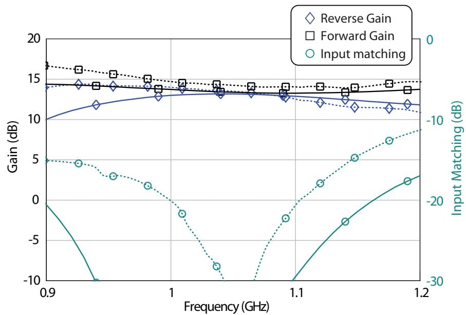
Figure 4.8: Simulated (solid line) and measured (dashed line) small signal gain (forward and reverse) and input matching for a 3-stage CRLH-TL-based distributed amplifier ( $I_{DS} = 30mA$ ;  $V_{DS} = 3V$ )
