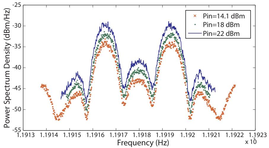
Figure C.5: Measured Power Spectrum Density for different input power (rms) levels.
