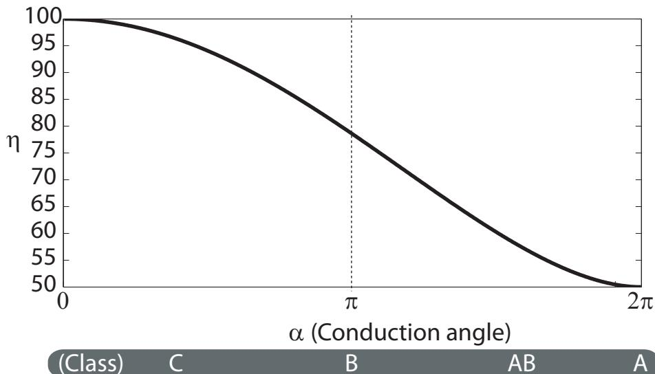
Figure 5.6: Drain efficiency,  $\eta$ , normalized to the corresponding Class A drain efficiency, as a function of the conduction angle,  $\alpha$ .
