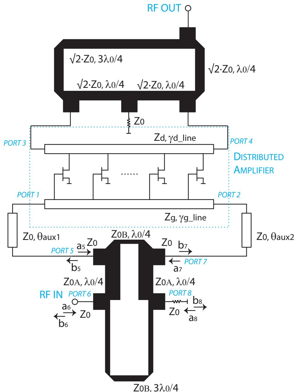
Figure 3.1:  $180^\circ$ -based implementation of the power recycling distributed amplifier
