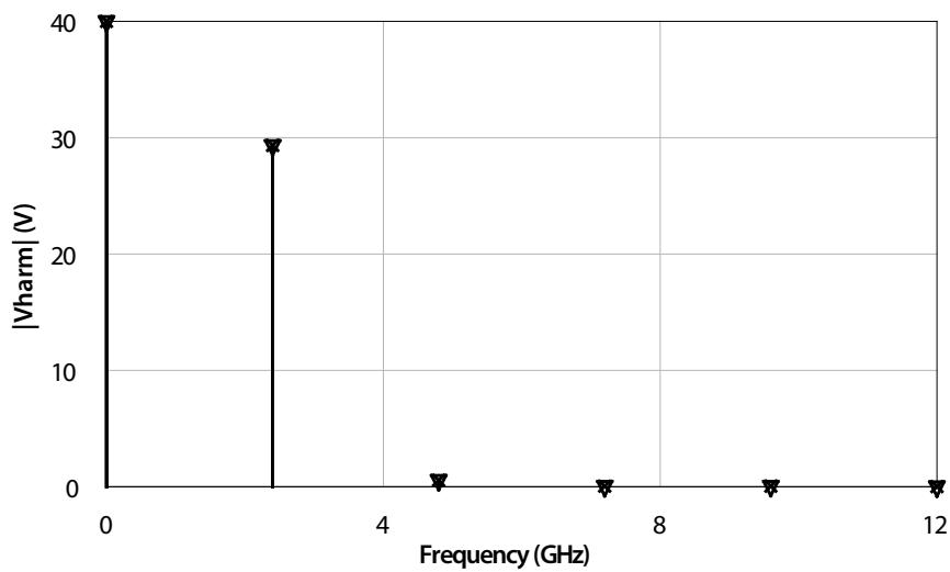
Figure 5.27: Harmonic components for the voltage for a 3-stage Class AB distributed power amplifier with output power combination ( $P_{in} = 18dBm$ )
