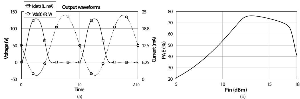
Figure 5.20: Theoretical output waveforms (a) and power added efficiency (b) for a Class B distributed power amplifier @  $f_0$  ( $I_{DS} = 0.067mA$ ,  $V_{DS} = 12.5V$ ).
