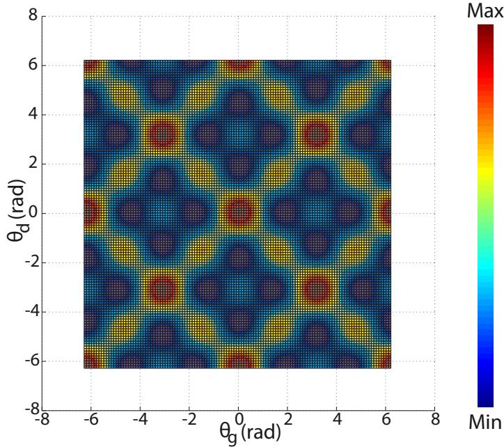
Figure 2.9: Normalized power delivered by the 3<sup>rd</sup>-stage of a 5-stage distributed amplifier as a function of gate and drain phase shifts (red areas represent maximum power values)
