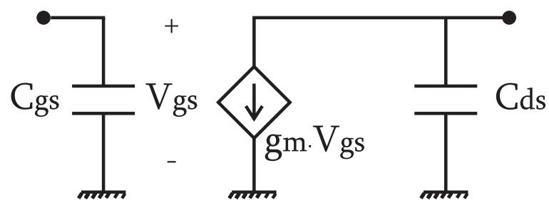
Figure 2.2: Simplified active device equivalent circuit
