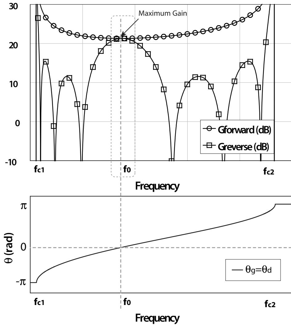
Figure 2.6: Forward and reverse gain of a 4-stage CRLH-TL-based distributed amplifier with identical gate and drain phase constants
