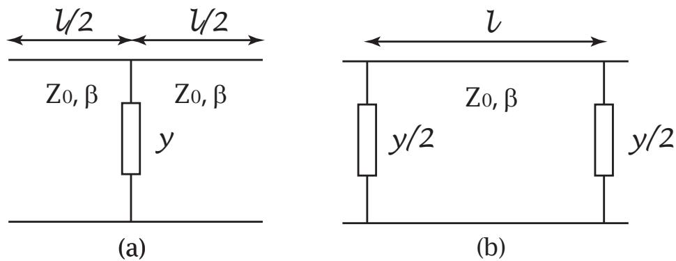
Figure A.12: Periodically loaded transmission line unit cell with (a)  $T$ - or (b)  $\pi$ -Topology
