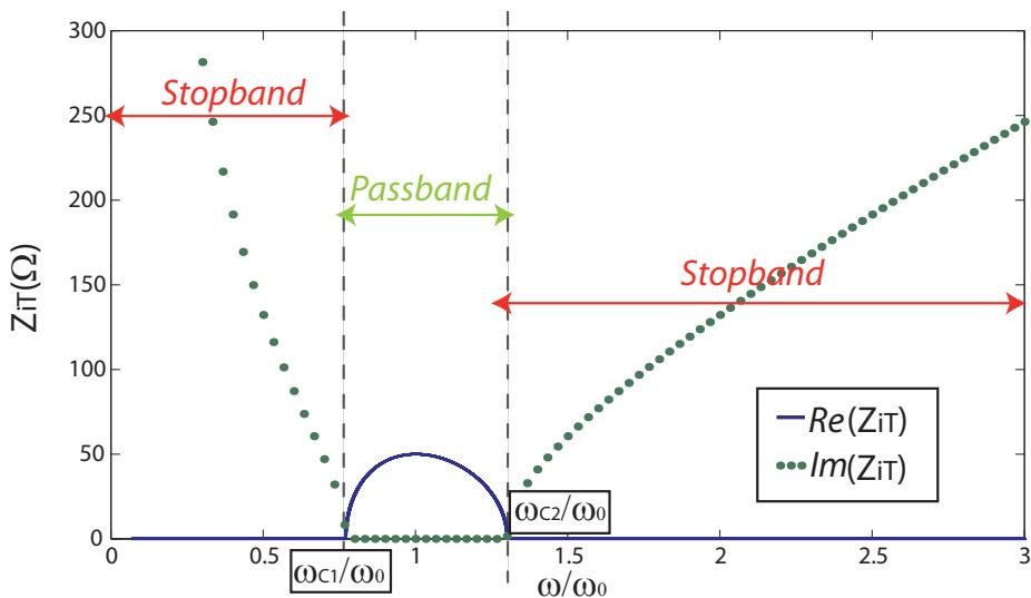
Figure A.8: Image impedance of a CRLH-TL unit cell with  $T$ -topology
