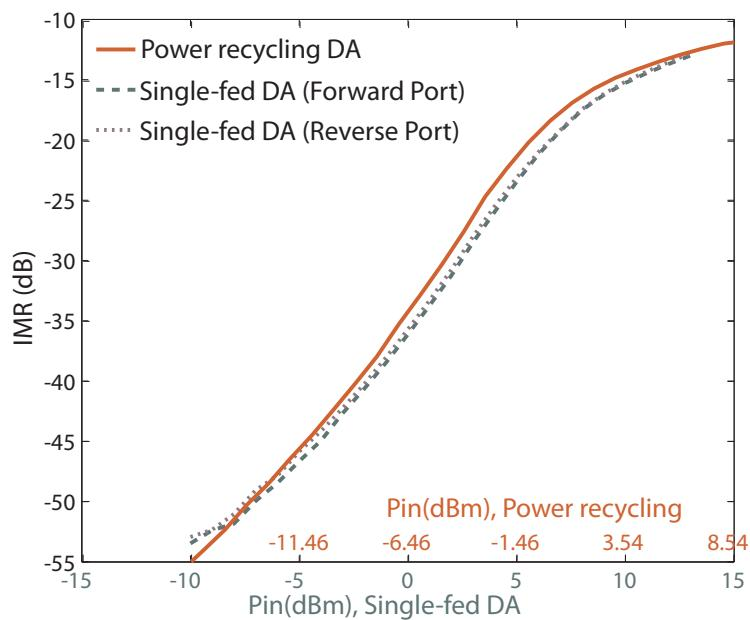
Figure 4.12: Comparison of the measured intermodulation distortion ratio of the power recycling DA versus the single-fed DA ( $I_{DS} = 30mA$ ,  $V_{DS} = 3V$ , two-tone test  $\Delta f = 1MHz$ ,  $f_0 = 1.07GHz$ )
