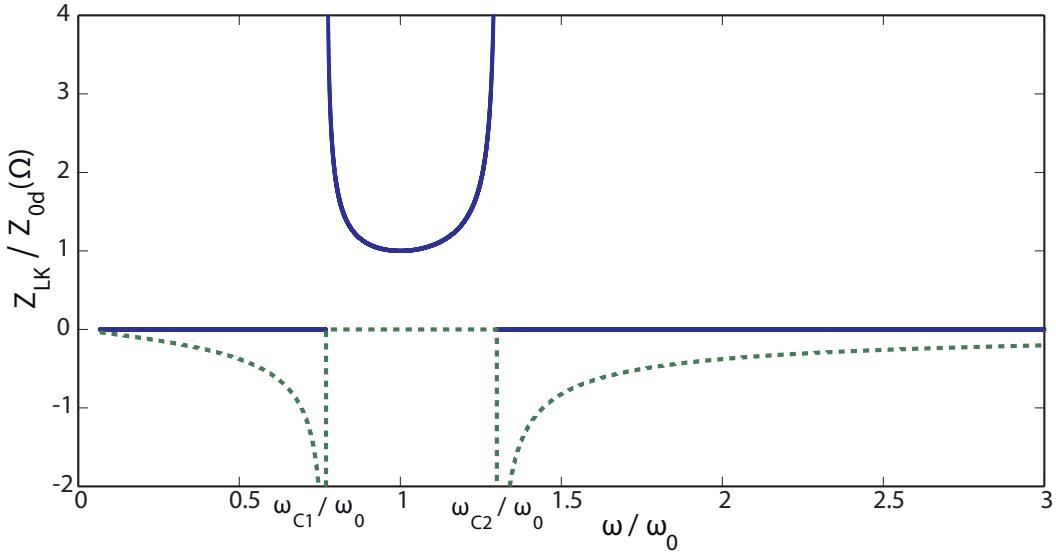
Figure 5.15: Image impedance of the drain unit cell (CRLH-TLs) with  $\pi$ -topology
