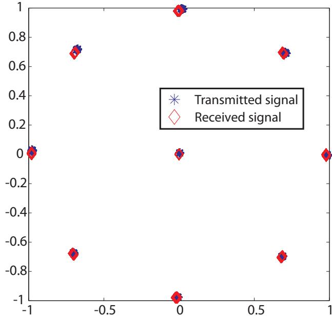
Figure C.8: Normalized Galileo's E5 signal constellation ( $P_{in}=24$  dBm).
