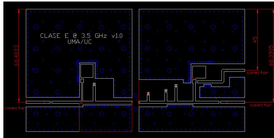
Figure C.18: Final layout of the designed Class E power amplifier for 3.5 GHz
