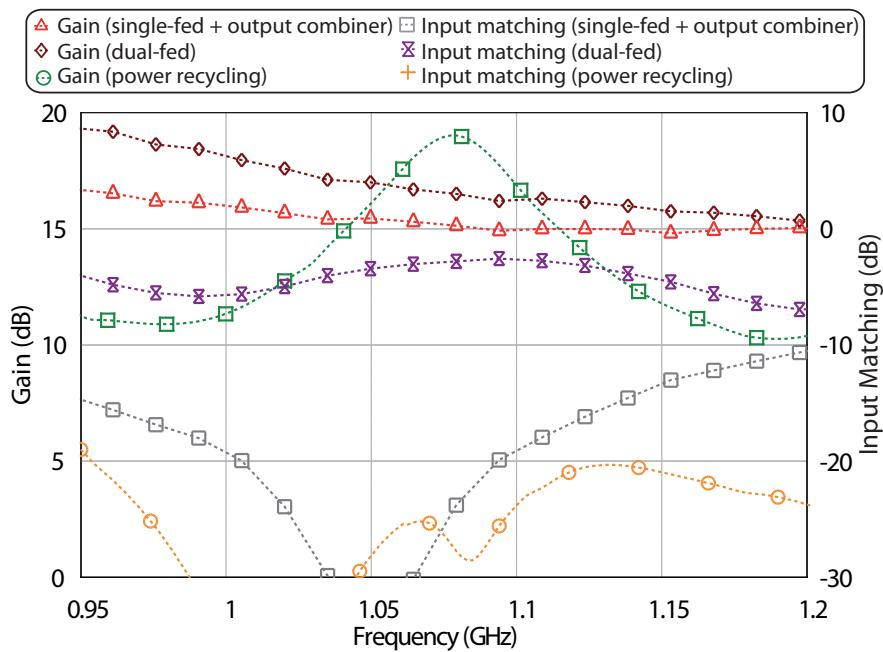
Figure 4.10: Measured small signal gain and input matching for three different 3-stage CRLH-TL-based distributed amplifiers (Bias point:  $V_{DS} = 3V$ ;  $I_{DS} = 30mA$ )
