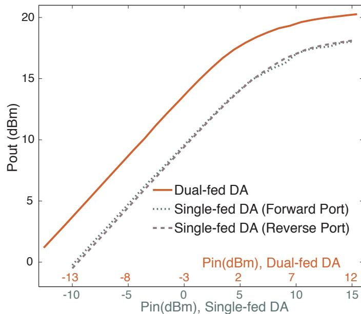
Figure 4.2: Measured Output Power @ 1GHz ( $V_{GS} = -0.3V, V_{DS} = 3V$ )
