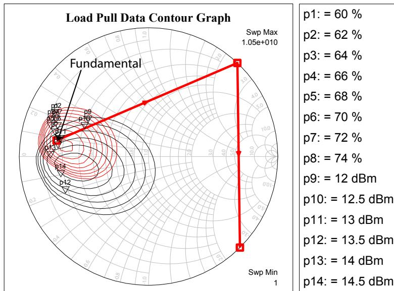
Figure C.14: Simulated load pull output power (black) and efficiency (red) contours for a GaN HEMT (Cree, CGH35015F) at the fundamental load of 3.5 GHz.
