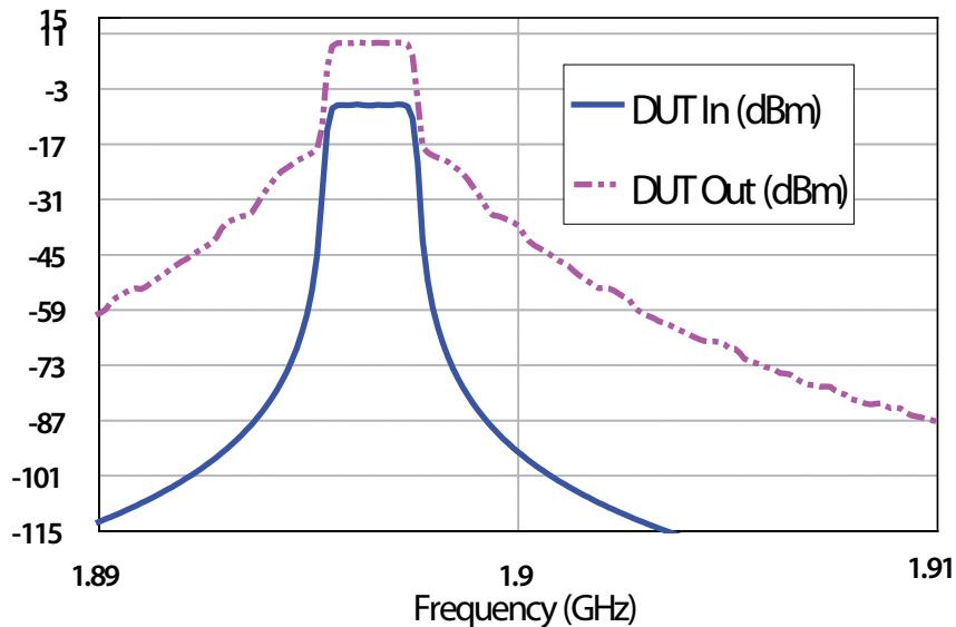
Figure 4.21: Simulated input and output power spectrum, LTE FDD signal @ 1.9 GHz.
