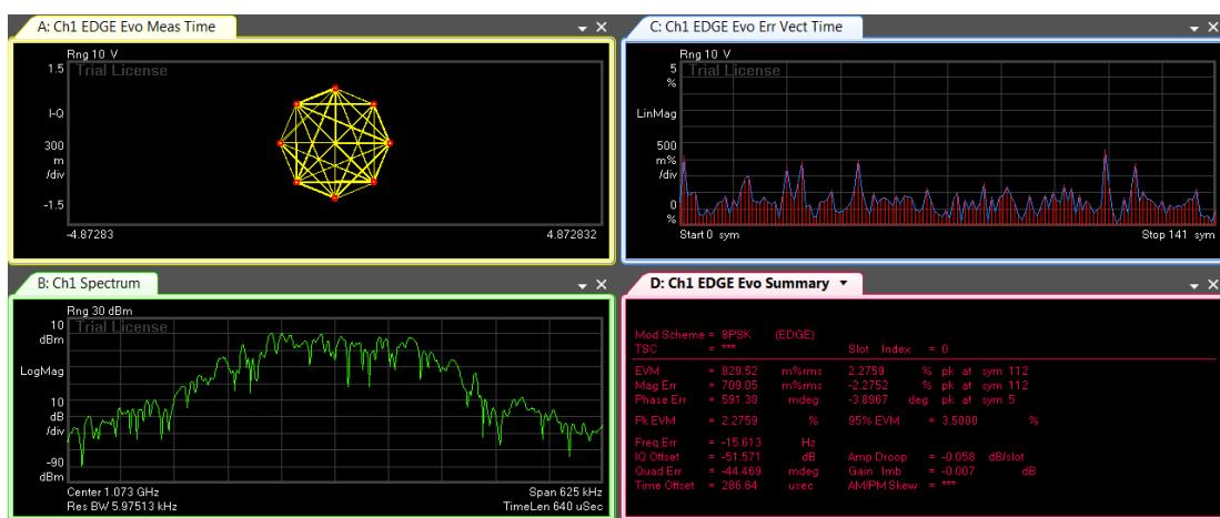
Figure 4.14: Amplified EDGE signal @ P1dB
